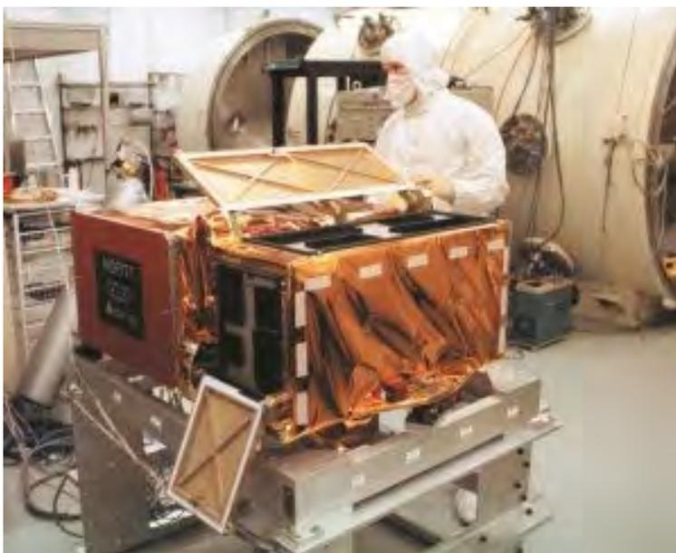
The MOPITT instrument undergoing test at the University of Toronto around 1995. (Photo credit: COMDEV)
