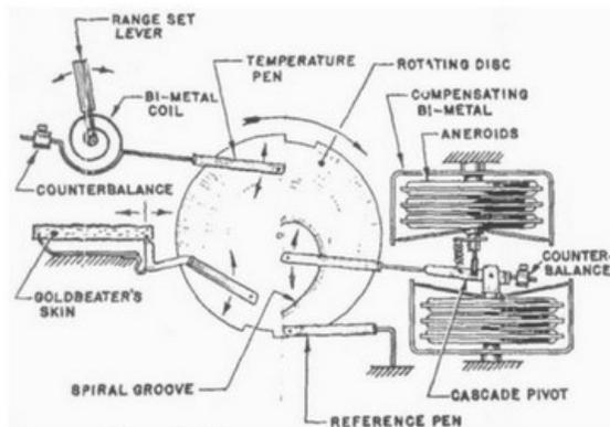
Figure 3: Chronometric Tethersonde (Bourke & Klein, 1967)
