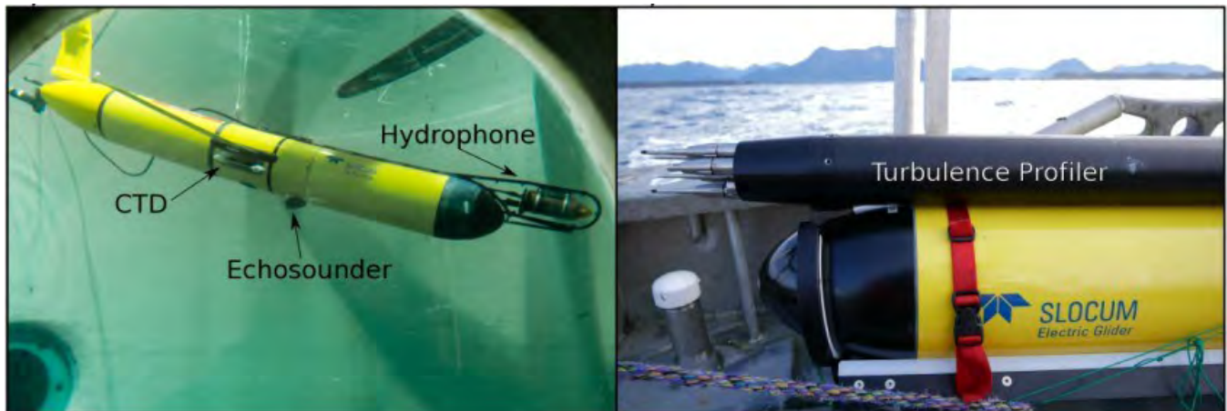
Figure 2: On left is the OTN glider with hydrophone, echosounder, and CTD shown. On right is the UBC glider with turbulence profiler shown.
